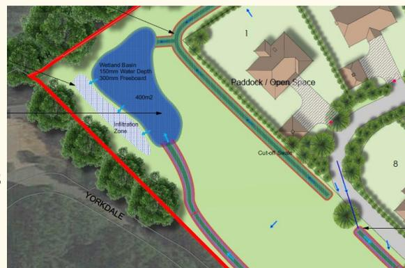
Long term monitoring and management was secured to control tree and scrub invasion, maintain water control structures - inflow and outflow, water level control, prevent unauthorised connections and changes to system, address any sedimentation and prevent invasive non-native species.
